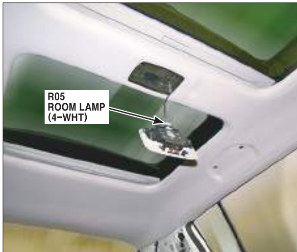
100. Center of Roof Trim
