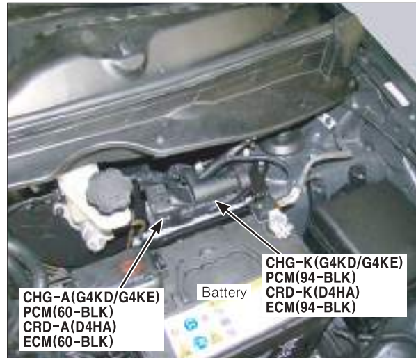
20. Left Rear of Engine Room
