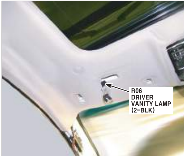
97. Left Front of Roof Trim
